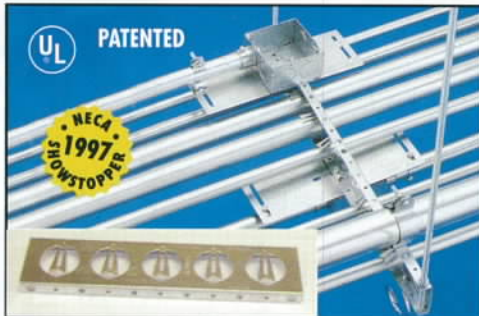
CONDUIT TRAPEZE BRACKET 1/2" thru 1-1/4", EMT, IMC or RIGID. Reduces labor—No conduit clamps required. Any length up thru 6 ft. maximum.
